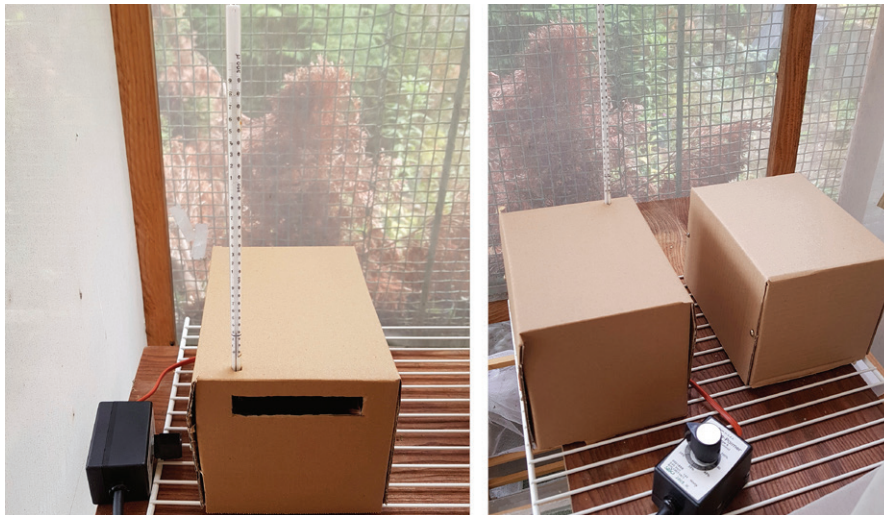
Fig. 1. Box shelters and experimental site. Heated box shelter (left). Heated and unheated (control) shelters (right).
